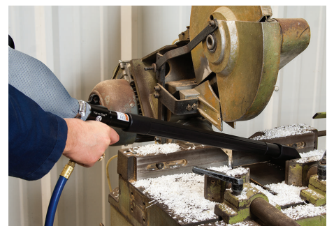
Model 6392 Vac-u-Gun All Purpose System removes plastic shavings from a saw.
