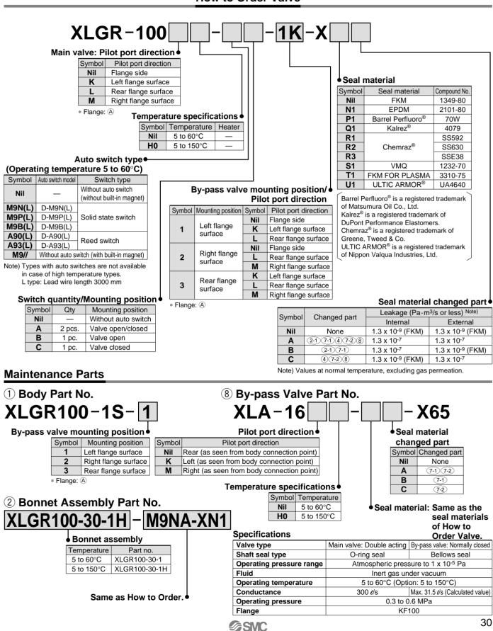
Aluminum High Vacuum Angle Valve/Double Acting/O-ring Seal Series XLG Made to Order 5
