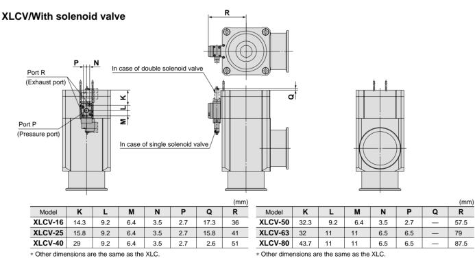
Note) For further details on solenoid valves, refer to the SMC solenoid valve catalog "SYJ3000/5000/7000" (ES11-84).
