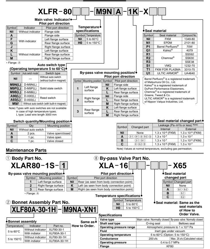
Aluminum High Vacuum Angle Valve/Normally Closed/O-ring Seal Series XLF Made to Order 2
