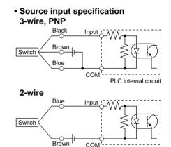
Connect according to the applicable PLC input specifications, since the connection method will vary depending on the PLC input specifications.
