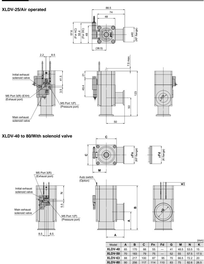
Note) For further details on solenoid valves, refer to the SMC solenoid valve catalog "SY100" (Best Pneumatics 2004 Vol. 4) and "SYJ300/500/700" (ES11-86).
