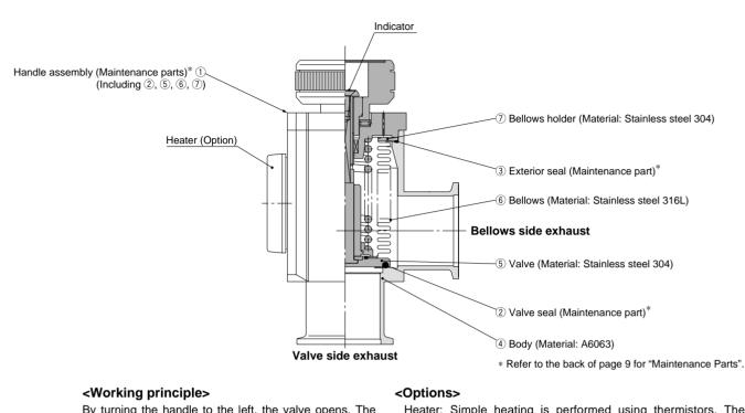
By turning the handle to the left, the valve opens. The handle does not move up and down, but the indicator shows the open or closed position of the valve. As the handle is turned to the right, the valve closes, and when the turning force of the handle suddenly ceases to be felt, the valve is sealed. The sealing force for the valve comes from the spring, and is constant.
